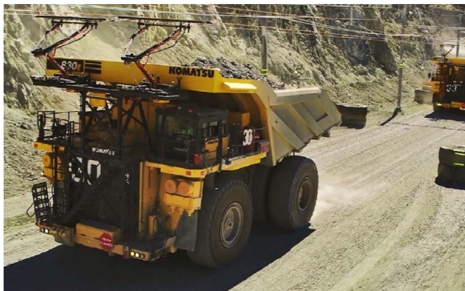
Electrification is key to decarbonization, so the industry is developing critical technologies such as charging stations and trolley systems for mining trucks. In Chile, for example, ABB is collaborating with mining companies and truck manufacturers to navigate the complexities associated with transitioning to fully electric mining operations. A first project, similar to the e-trucks shown here in a copper mountain mine in Canada, is expected to be completed by early 2025.
